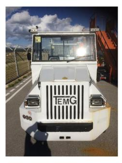
ENGINE: Diesel Deutz F4L912 model aircooled. 4 cylinders. Diameter/path: 100/120 mm. Charge: 3770 litres. Relation of compression: 18. Max. power: 54 KW/2500 r.p.m. Torque engine max.: 247 Nm to 1450 r.p.m.
