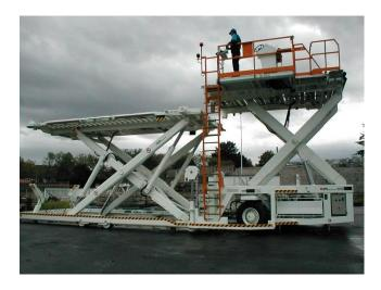
Solid wheels modules for independent load transfer on the front, middle and rear parts of the main platform.
