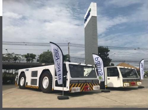
The Bliss-Fox F1-300 Aircraft Tractor was designed in Australia for both pushback and extended towing of aircraft up to 360 Tonnes. Drop-in ballast in the F1-300 easily transforms the tractor from a standard 27 Tonnes for A330 & B787 up to 40 Tonnes for A350 &B777 with no obstruction to the operators' line-of-sight.
